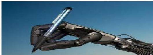
Figure 4. The Utah/MIT Dextrous Robotic Hand
